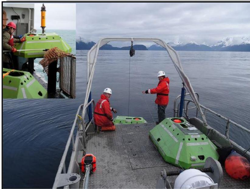
Mooring assembly composed of green trawl-resistant cover and instruments inside, which weigh about 850 pounds with a 1-inch thick plate steel anchor as the base. Photo courtesy: NOAA/AFSC.
